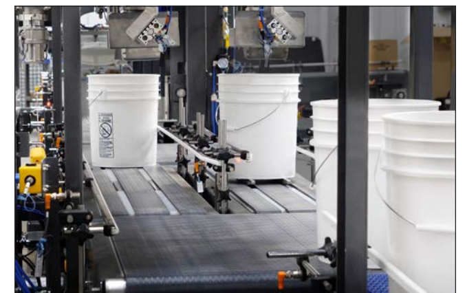
BULK CONTAINER FILLING: CONTINUOUS MULTI-LANE
