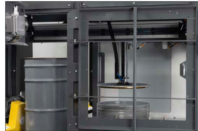
DRUM LID ALIGNMENT: PICK-AND-PLACE
