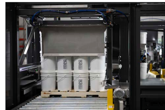
PALLETIZING: LOAD STABILIZER
