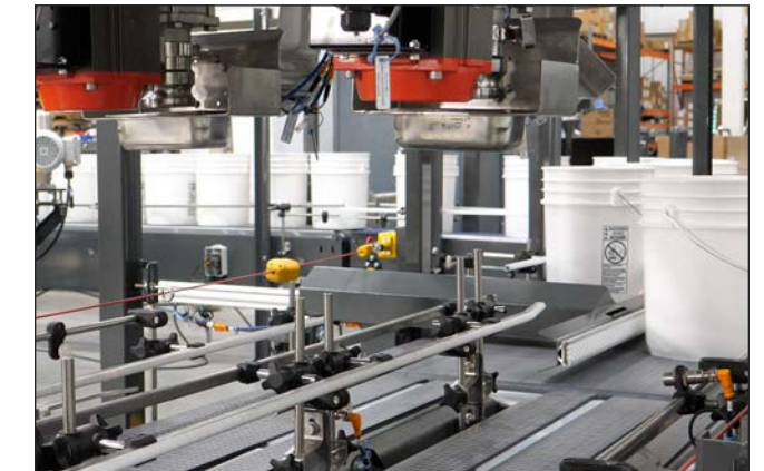
PAIL ALIGNMENT GUIDES & STOPS
