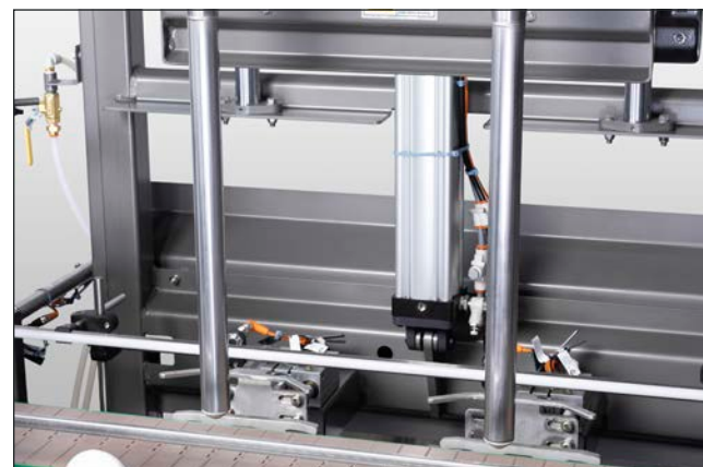
CARBON STEEL FRAMEWORK FINISHED TO FDA STANDARDS
