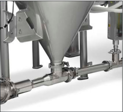
Clean-design Engineering & Construction: Reduce changeover times and increase cleaning efficiency. Sanitary clamp fittings are engineered into system assemblies to aid disassembly and reassembly.
