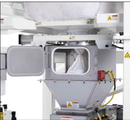
Bag Spout Untie Box: Contain material with an enclosed bag spout. Integrated flow control valve and application-specific downstream interconnect enable effective material discharge and supply. Toggle-action door handle provides dust-tight seal.
