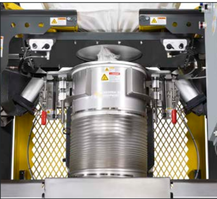
Pinch Valve: Pneumatically actuated blades compress bag spout to break-up and release large chunks of material that may slow flow rate. Can close through static column of material for partial bag unloading. Actuated using a two-handed pneumatic safety control circuit.
