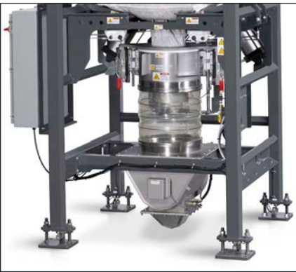
Bulk Bag Empty Alert System: Support continuous operation with bag empty visual alerts. Loss-in-weight scales, engineered into the framework, gauge net-weight loss during material discharge. Operator alerts occur when scales reach customizable target weight.
