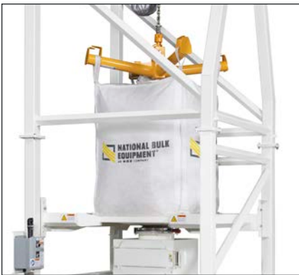
Bulk Bag Support Pan: Maintain bulk bag stability and bag spout alignment during discharge of free-flowing materials. Sloped bag support pan directs material toward bag spout interface; enables safe operator access to bulk bag discharge spout.
