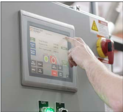
Controls & Automation: Customized programming along with components provide safety features to prevent unwanted operator interactions. Integration of grounding monitor, audible and visual alarms, interlocking switches, and level sensors ensure operators follow proper sequences.
