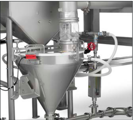
Slurry & Solution Material Supply and Processing: Deliver precise, homogeneous concentrations to downstream processes. Controlled discharge, metered infeed, and proper blending of dry solids into the liquid supply enables optimal throughput and yield.
