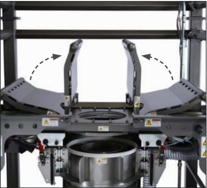
Pneumatically Actuated Massage Paddles: Reliable, consistent discharge of non-free flowing material is made possible by simultaneous upward and inward motions of the massage paddles, causing a gradual displacement of material toward the bag spout.
