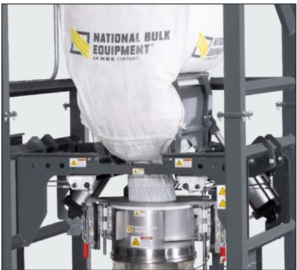
Pneumatically Actuated Massage Paddles: Increase material discharge rate, maximize discharge of material from the bulk bag. Based on downstream signals, massage paddles direct material from far-corner areas of bulk bag toward discharge spout.
