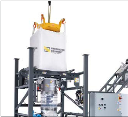
Customer-supplied Bag Loading System: Optimize existing crane and hoist systems; ensure effective bulk bag loading. Lower-frame only bag support systems enable safe operator interaction. A variety of bag spout interface methods aid material discharge.
