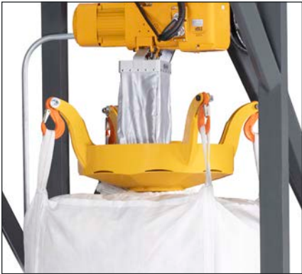
Low-profile Bag Hanger: Reduce total equipment height and enable integration of application-specific sub-assemblies. Raised bag hanger arms, offset from the contaminant guard, optimize bag hanging height and reduce headroom requirements.
