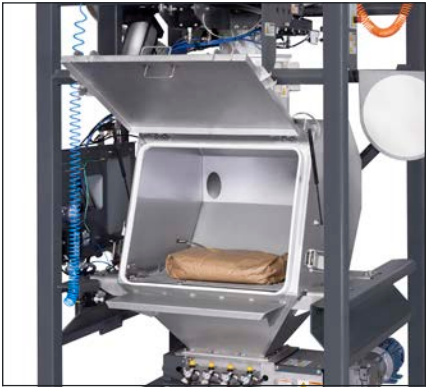
Combination Hopper: Enable manual addition of ingredients from alternate containers in an ergonomic workstation with bag grate and interlocked door. Integrated baffles inside the hopper allow for dust collection to draw the dust down into the system and away from the operator.
