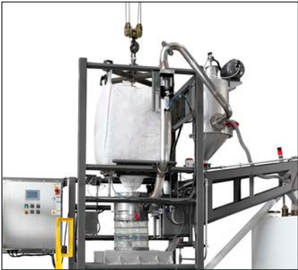
Customer-supplied Bag Loading System: Utilize facility hoist and crane systems for bulk bag handling and loading into the lower-frame only bag support system. Application-specific bag spout interface enables safe, easy access for operator; prevents dust release.
