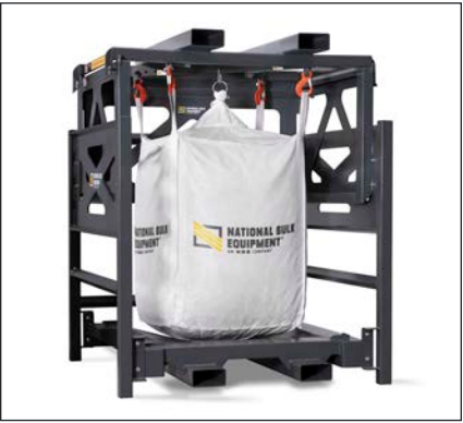
Split Frame: Improve bulk bag loading effectiveness in low-volume supply applications. Two-part framework and loading sequence reduce overall raised height required of forklift and enables forklift loading in low-headroom locations.
