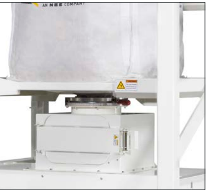
Iris-type Valve: Designed for use with free-flowing materials, the iris-type flow control valve enables gradual start-up of flow. Manage material flow volume through the bulk bag spout and protect operator's hands from material contact during untying of spout.
