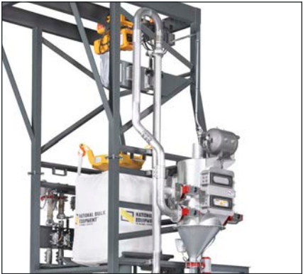
Enclosed Dust Recovery System with Air Balance Actuation: Prevent over-pressurized discharge of material with fluid-like flow by locating the vent stack above the bag height; avoid dust release into work area. Auto-actuated air flow volume controller uses make-up air to balance air circuit during discharge.
