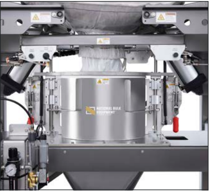
E2™ Bag Spout Interface: Ensure secure, enclosed interface of bulk bag spout to downstream process; prevent spout release during material conditioning and discharge. Dust-tight seal prevents material loss and additional clean-up due to fugitive dust. Additional cover prevents dusting during minor adds.
