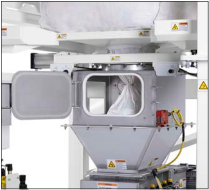
Bag Spout Untie Box: Provide effective access to enclosed bag spout and ties. Integrated flow control valve and application-specific downstream interconnect aid material discharge and supply. Optional view window provides safe visibility of discharge status.
