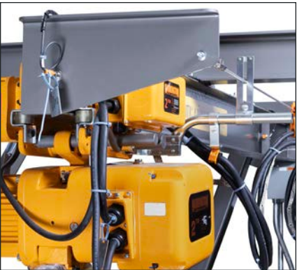
Bulk Bag Loading Location Sensors: Enable designed operator interactions for proper loading and handling of bulk bags. Sensors placed along bag support framework rail detect trolley and hoist location to enable or disable local and remote hoist controls.
