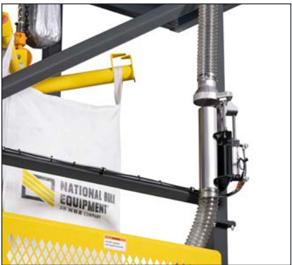
Integrated Dust Collection System with Actuated Vent Stack: Avoid loss of material to dusting and unwanted material entrainment during dust collection. Auto-modulation of pick-up air at spout interface reduces product loss during material discharge.
