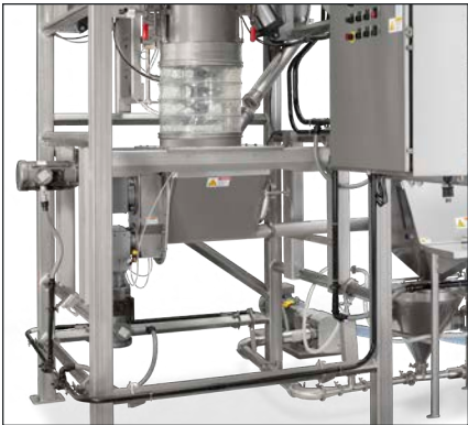
PVC-coated Rigid Conduit Runs: Protect system-wide controls, sensing, and monitoring wiring from corrosive process environments and materials. Application-based conduit material specifications and routing design extend system availability and reduce maintenance. Galvanized, aluminum, or stainless steel conduit is available.
