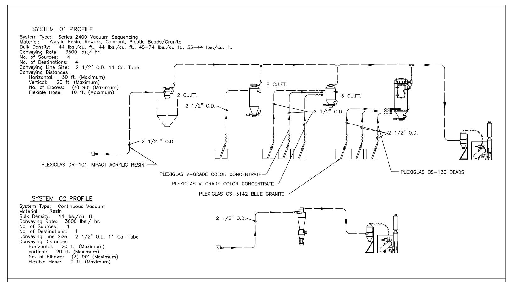
Equipment was purchased through an OEM and installed at end user for producing plastic pellets. Raw material is conveyed from silos and Gaylord boxes. The receivers discharge in loss-in-weight screw feeders. The feeders discharge into an extruder. The extruder discharges into a cooling bed of water. The strand is then cut into pellets. The pellets are conveyed to a cyclone and fed by an Aerolock into a Gaylord box.
