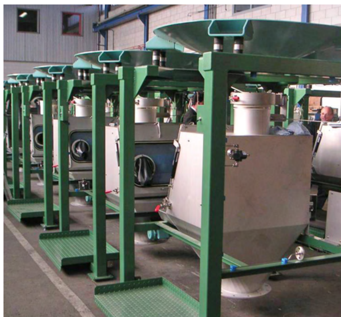
Bulk bag unloading stations combined with bag emptying stations for a PE Plant
