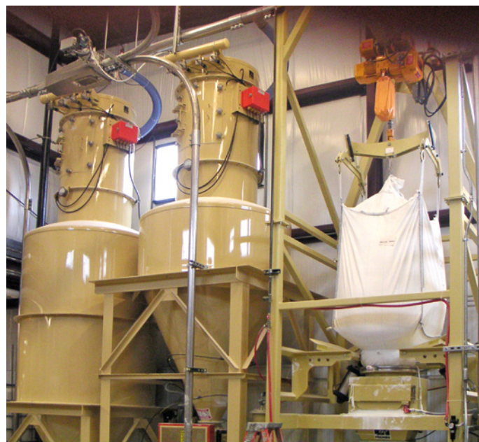
A Coperion K-Tron continuous vacuum system receiving \text{TiO}_2 from a bulk bag unloader and filler from a receiver/surge hopper into a scale hopper.
