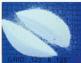
Spherical, irregular particle shape with adhesion on impact areas and potential for flooding characteristic
