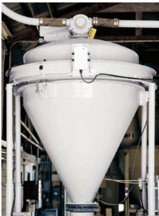
Scale hopper with Aeropass valve at top
