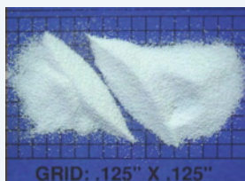
Irregular particle shape with static adhesive, fluidizable and dusty characteristics
