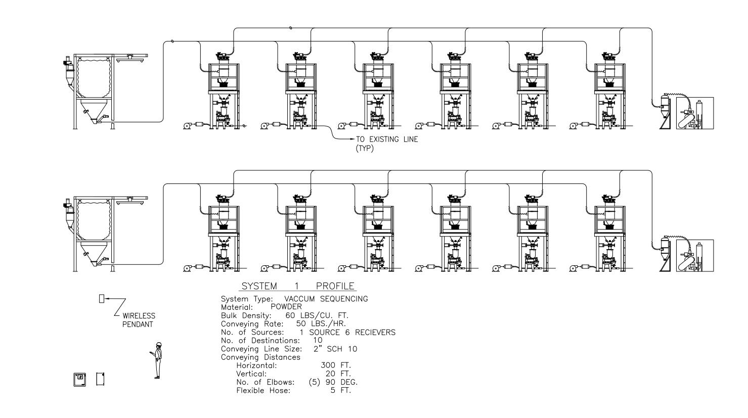
Two separate conveying systems for conveying SAP in the manufacture of diapers. Each system has 6 receivers. The convey rate to each receiver is under 100 pounds per hour. The source of each convey system is a bulk bag unloader with trolley and hoist with an integral dust collection system.
