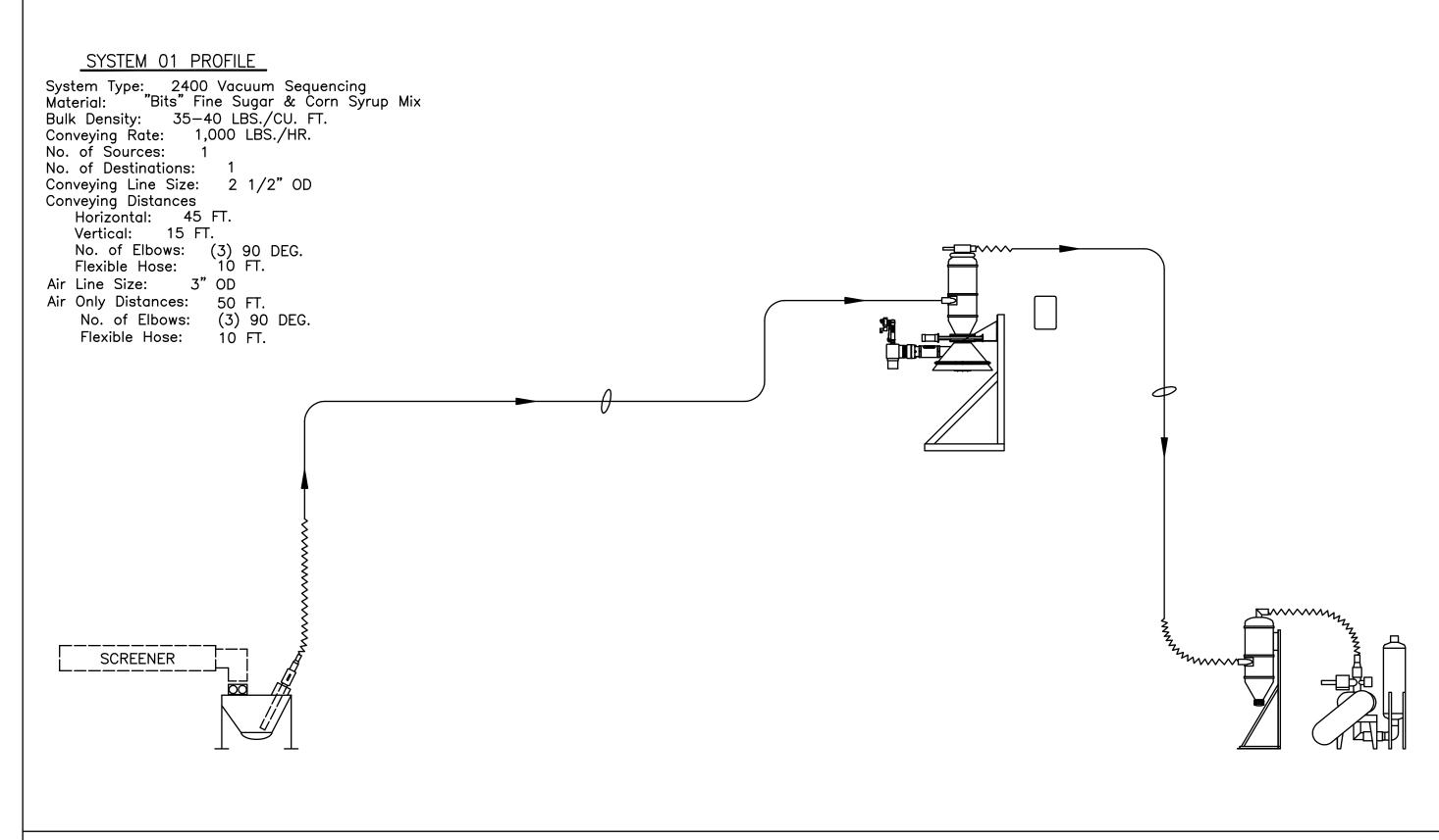
This project was for a food seasonings producer. This system involved a vacuum sequencing system to load fine sugar and corn syrup mixes in different flavors from the outlet of a screener to load small tray containers. Design includes unique dust collection apparatus on the outlet of receiver to cut down on dust during dump from the receiver discharge.
