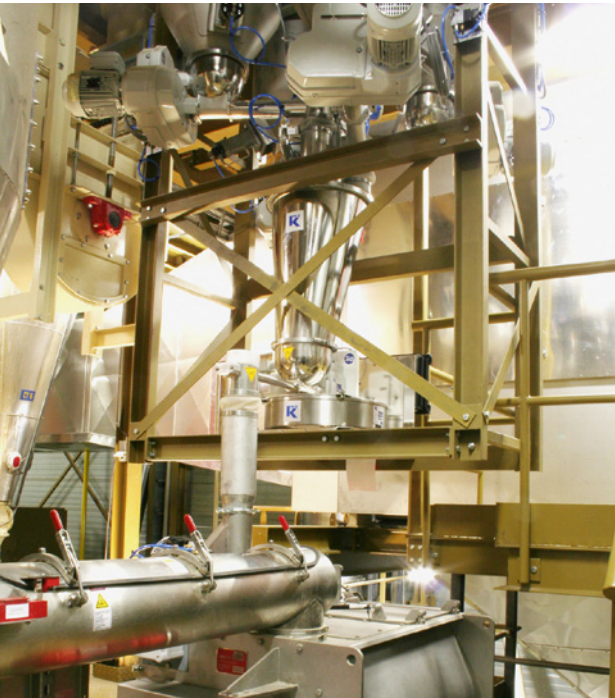
Loss-in-weight screw feeder feeding into a mixer
