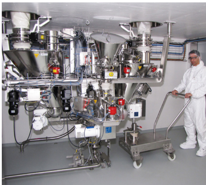
Photo 7: Multi feeder continuous infant formula production complete with integrated off-line scale for feeder sampling, validation and calibration.
