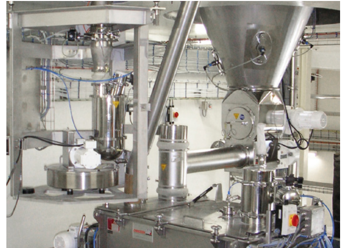
Photo 1: Coperion K-Tron feeders over a continuous mixer
