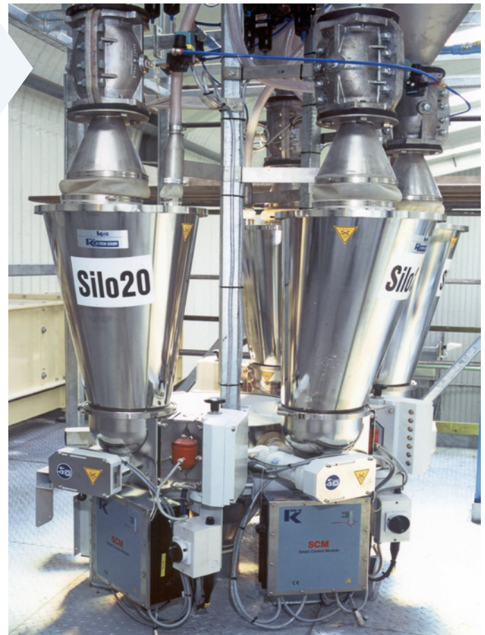
K2G Loss-in-weight feeders are mounted in carousel fashion. These units meter enzymes.
