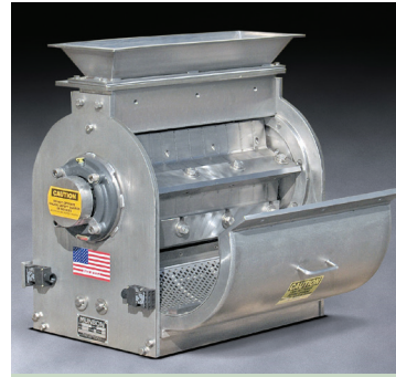
Sanitary Stainless Steel Rotary Knife Cutter with large clamshell doors on both sides allows thorough wash down between runs of multiple materials, preventing cross contamination. (Shown without drive components or support base for pneumatic collection).
