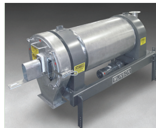
Rotary Continuous Mixer shown with ASME-code high pressure jacket for heating or cooling with water, steam or oil.
