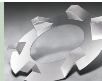
Solid "weirs" at the discharge end of the mixing drum function as a dam to build a "residence volume" of material before it overflows the weir. For applications requiring complete clean-out, an optional "discharging weir" (shown) scoops remaining material from the drum when its rotation is reversed.
