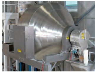
A food processing plant uses this 140 cu ft (4 m 3 ) capacity, sanitary Rotary Batch Mixer. Complete evacuation allows fast, thorough cleaning between batches with minimal downtime.
