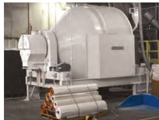
This industrial grade, 300 cu ft (8.5 m 3 ) capacity Rotary Batch Mixer blends recycled PVC films with colorants and other additives for salable products.
