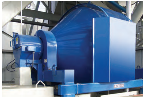
This 90 cu ft (2.5 m 3 ) abrasion-resistant Rotary Batch Mixer blends dry cement mixes in less than three minutes, gently and efficiently with total uniformity.
