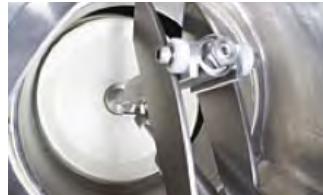
Exterior view of plug gate discharge valve in open position.
