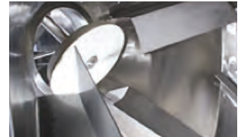
Interior view of rotating stainless steel mixing drum showing plug gate discharge valve pivoted to the open position, and mixing flights that blend and elevate bulk material.
