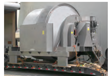
This Rotary Batch Mixer with #316L stainless steel product contacts operates with equal efficiency loaded with 400 cu ft (11 m 3 ) of drink mixes down to 20 cu ft (0.6 m 3 ).
