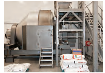
At a major contract manufacturer of nutritional supplements, this MUNSON® 300 cu ft (8.5 m 3 ) capacity Rotary Batch Mixer handles whey, soy, protein and greens, as well as sugar- and fructose-based powders, with no cross contamination.
