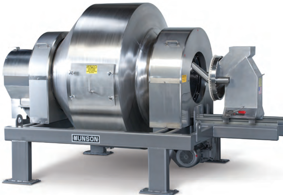
Rotary Batch Mixers are available in useable capacities to 600 cu ft (17 m 3 ). Shown is a 40 cu ft (1.13 m 3 ) sanitary stainless steel model with retractable inlet, for blending of spices.
