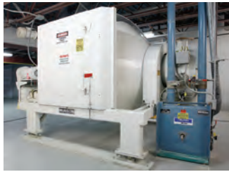
50 cu ft (1.42 m 3 ) capacity Rotary Batch Mixer at one of the world's largest producers of pesticides ensures uniform distribution of a liquid addition on a carrier.
