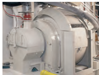
Over 300 different glass compositions, each containing 5 to 15 ingredients, are blended in this abrasion-resistant Rotary Batch Mixer with no cross contamination.
