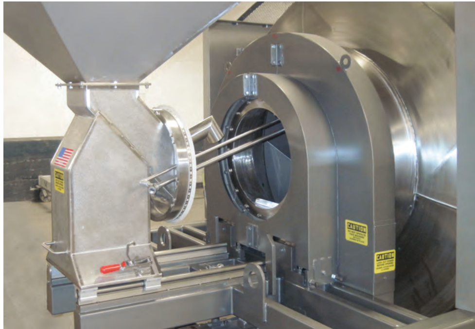
The sliding intake chute of the Rotary Batch Mixer shown in the open position, allows rapid access to the drum interior as well as the intake spout and seal area for cleaning and inspection.
