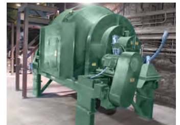
This 300 cu ft (8.5 m 3 ) XHD Series Rotary Batch Mixer blends batches of metal powders ranging from 22.5 tons down to 2.25 tons with equal efficiency.
