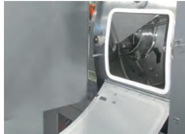
Large doors provide unrestricted access to the wide-open vessel interior for cleaning and inspection.
