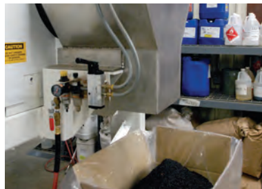
Rotary Batch Mixer shown discharging one of 200 blends of tea with no cross contamination.
