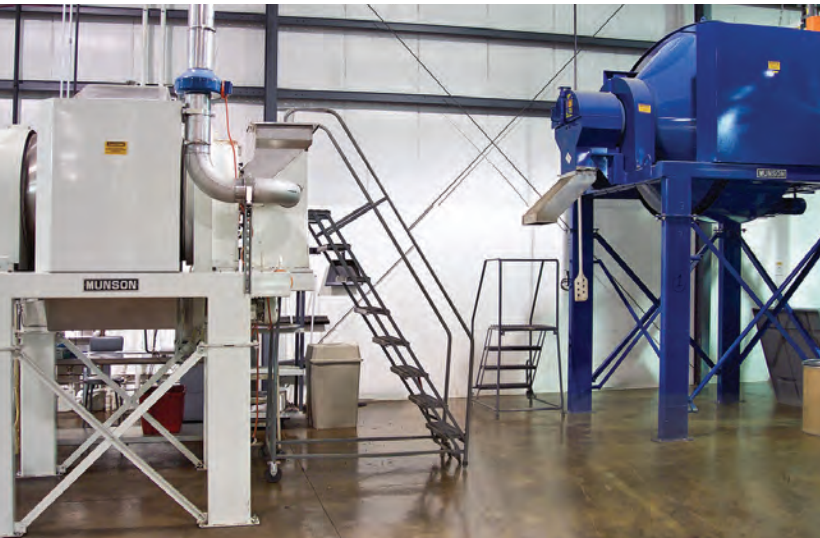
25 cu ft (0.7 m 3 ) MUNSON® stainless steel Rotary Batch Mixer (left) and 50 cu ft (1.4 m 3 ) carbon steel Rotary Batch Mixer at a leading coffee processor.
