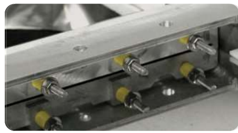
PTFE-treated bonnet packing gland, for greater wear resistance and longer service life
