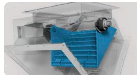
Optional “rock box” liners allow materials to collect and abrade upon themselves, rather than continuously abrading upon the diverter’s material contact areas
