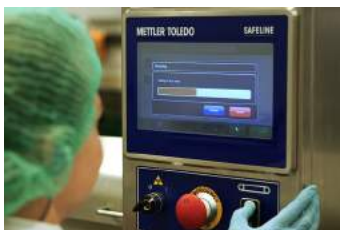
Figure 3: Maximum permitted leakage levels from an x-ray system = 1 \mu Sv/hour (ROW regulations), 5 \mu Sv/hour (US regulations)
