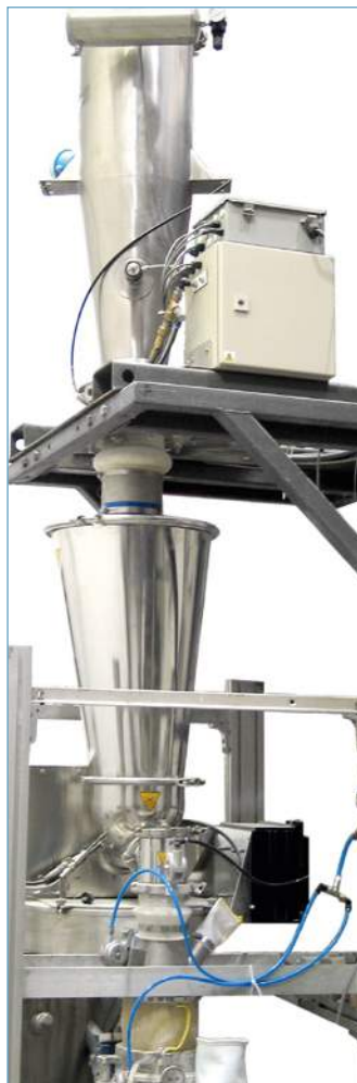
Pneumatic refill receiver above Coperion K-Tron LIW feeder
