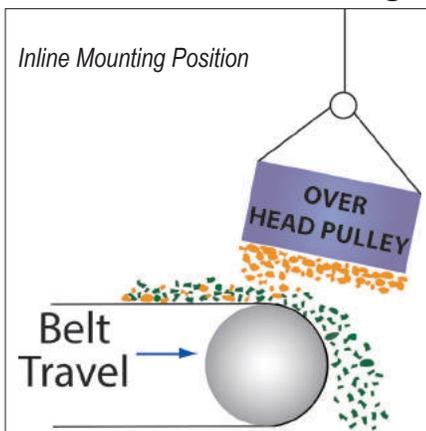
**Inline installation is preferred** because magnet separation efficiency is at its best when magnet is located over where conveyed material opens up during its path through air
