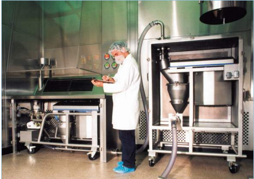
Conveying in-line through two mills, the first as a deagglomerator and the second for finer particle size
