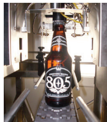
A bottle of beer with crown cap passes under the RTV-AC sensor.
