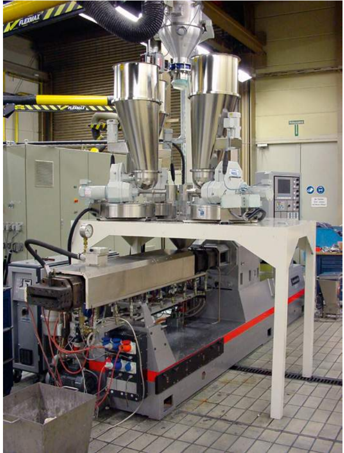
Coperion K-Tron feeders with refill system on a compounder
