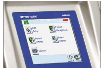
PowerPhasePRO systems feature a large, full color touch screen interface with an icon driven menu.
