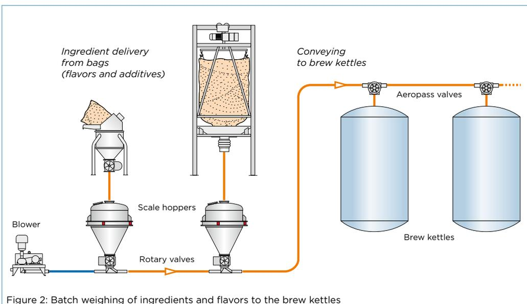
Figure 2: Batch weighing of ingredients and flavors to the brew kettles
