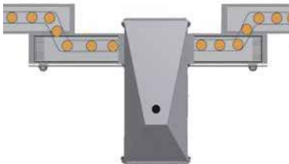
Figure 11: Offsetting the x-ray machine from the main production line removes the direct line of sight to the primary x-ray beam
