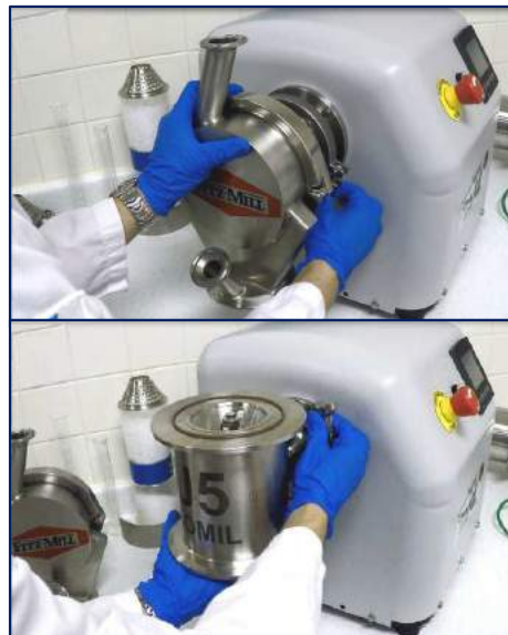
Figure 2: Interchangeable Milling Modules Via Sanitary Clamp Connection
