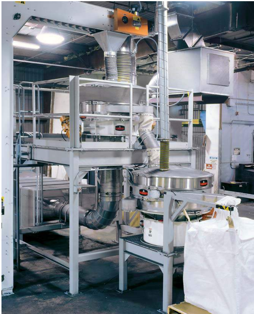
This skid-mounted, turnkey dryer-screener system configures a 48-inch (1220 mm) fluid bed dryer and two-deck circular vibratory screener in series to dry proprietary chemical powder while removing undersize and oversize particles at the rate of 2000 lbs/h (907 kg/h). The screener is equipped with a bulk bag hanger and extended discharge spout to align with the bag intake spout, and magnetic ferrule to remove tramp metal from the finished product prior to packaging.
