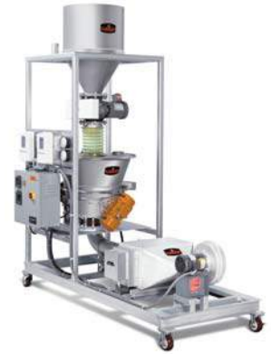
This pilot-plant-scale drying system incorporates a surge bin, rotary valve, 24" (600 mm) diameter fluid bed processor, heater, blower, and controls on a caster-mounted frame. Processors as small as 18" (450 mm) in diameter are offered for laboratory applications.
