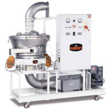
With simple connections to an existing dust collector and power source, this fluid bed dryer system is ready to reduce the moisture content of boric acid from 10 to 0.5 percent on a batch basis. It combines a 40" (1000 mm) diameter fluid bed processor, heater, blower, and controller on a caster-mounted skid.
