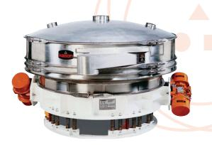
screen at high rates. The "Flo-Thru" Circular Screen Separator is designed for screening of dry materials and solid/liquid applications. Available from 18" to 84" (460mm to 2135mm) in diameter. Can be rated for positive pressures to 14.7 psig or negative pressures to 14 inches mercury.
