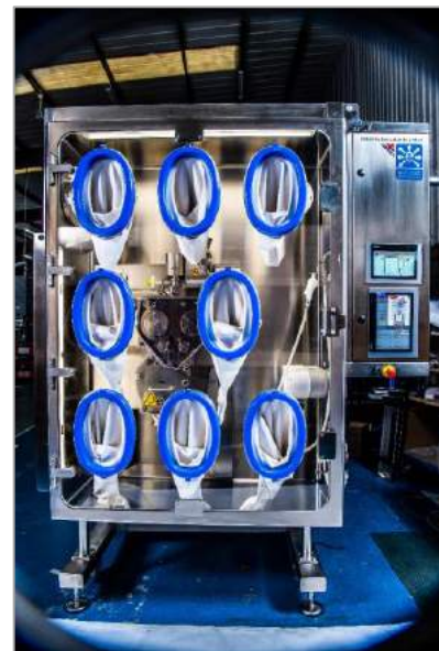
Complete isolator providing OEB 5 containment with integrated compactor
