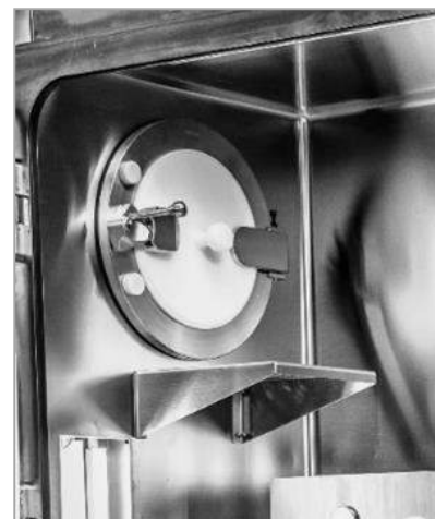
Entry Rapid Transfer Port (RTP)
