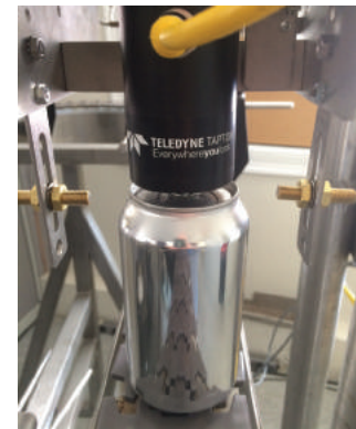
Beer Can Passing Through the TapTone Proximity Sensor
