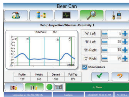
“Bad” Can on Proximity Sensor
