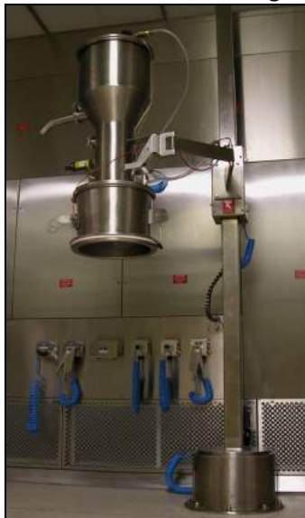
Figure 6: Quadro Vac® Pneumatic Conveying System equipped with an Earth Monitoring System
