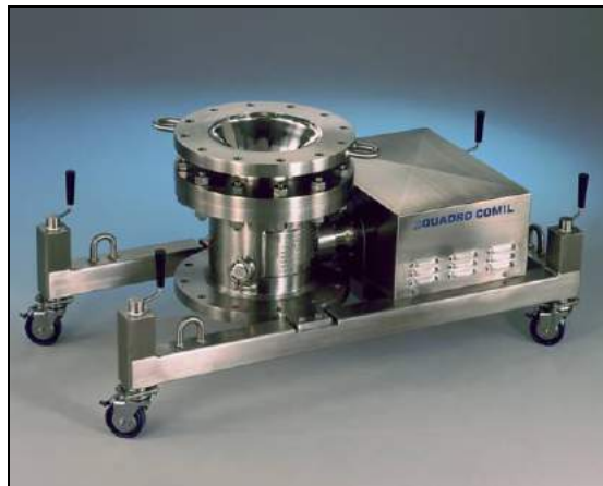
Figure 3: Explosion Pressure Shock-Resistant (PSR) Quadro® Comil®
