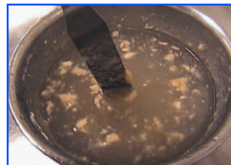
“Fisheye” Formation With A Conventional Mixer
