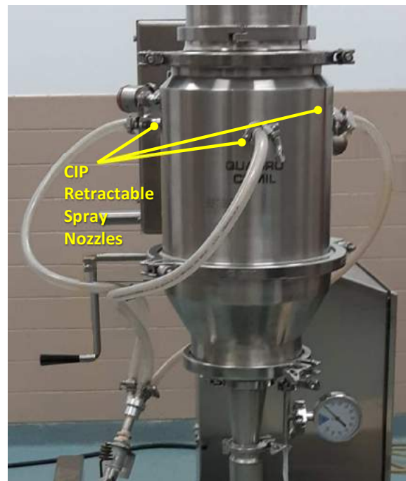
Fig 3: Comil® U20x CIP Test Set Up
