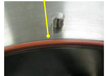
Fig 6: Housing O-Ring Detail CIP Cycle
